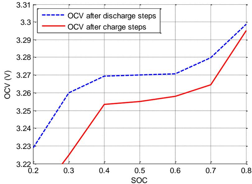
Figure 18. Experimental data on voltage  $U_{oc}$ , after discharge steps and after charge steps.
