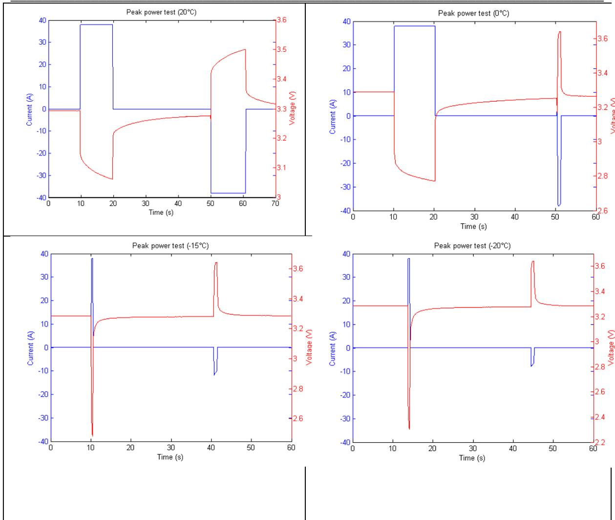
*Figure 3. Results of the peak power tests at different temperatures.*
