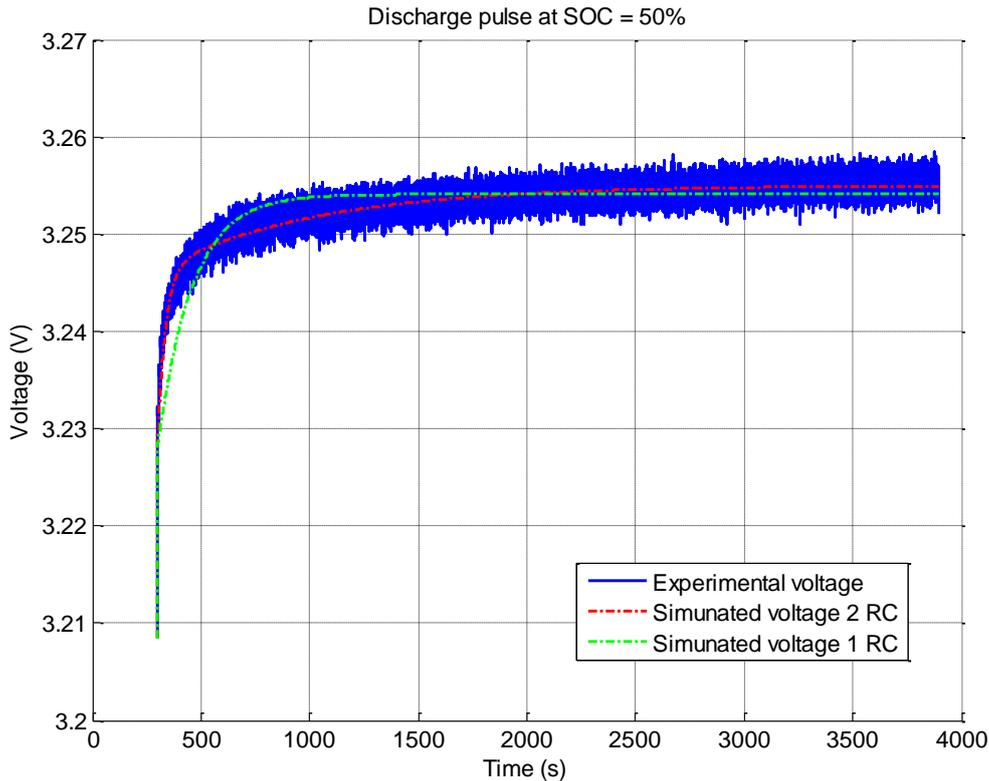
*Figure 5. Voltage behaviour immediately after the end of a discharge process, while SOC=50%.*
