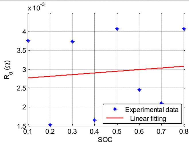
Figure 14. Experimental data on  $R_0$  and linear interpolation.
