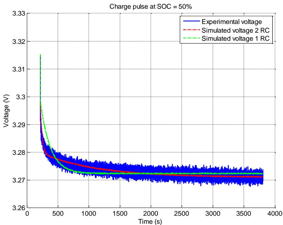
*Figure 9. Voltage behaviour immediately after the end of a charge process, while SOC=50%. Comparison between experiment and model ( $R$ 's,  $C$ 's,  $U_{oc}$  determined by error minimisation).*
