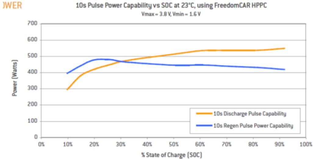
Figure 2. Power graph of the selected Li cell, supplied by the manufacturer.
