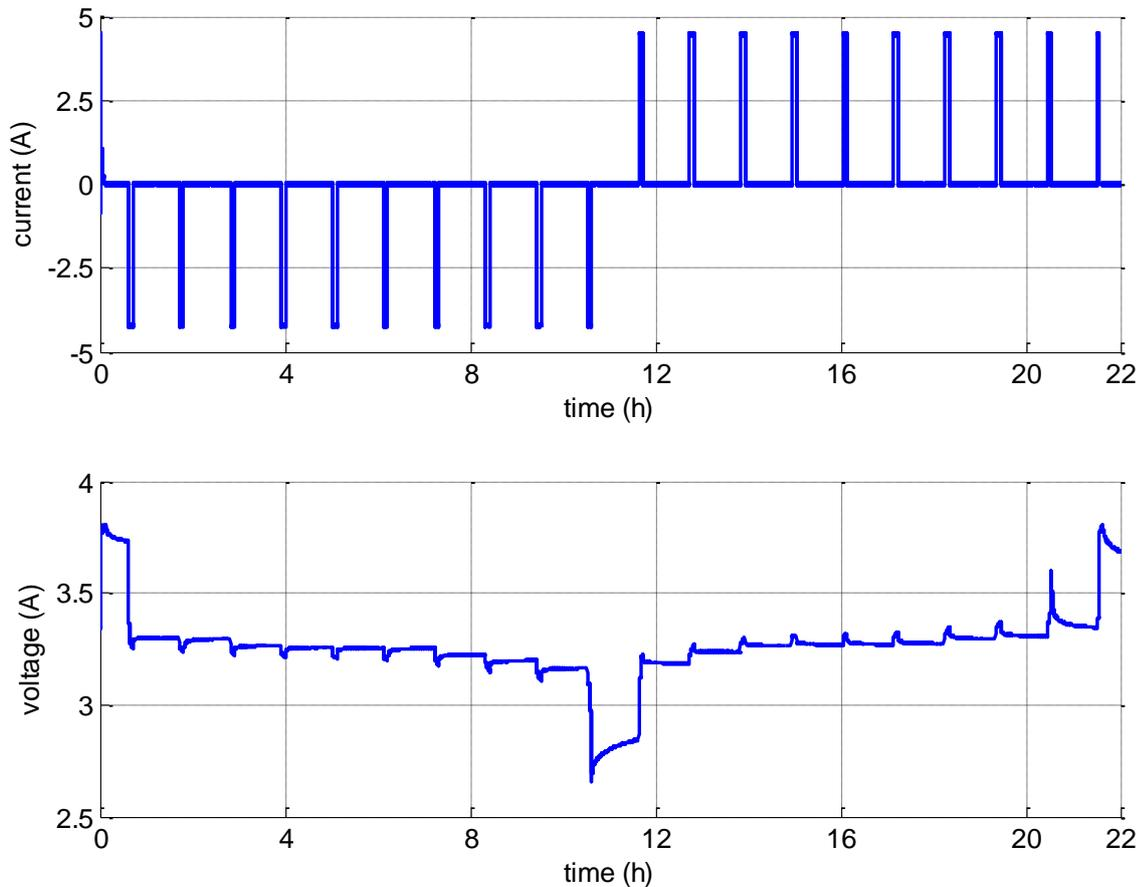
*Figure 13. Current (above) and voltage profiles as measured during MST: discharge-based (up to  $t=10$  h) and charge-based (above  $t=10$ h).*
