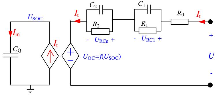
Figure 19. Cell model with 2 R-C blocks (form 2).
