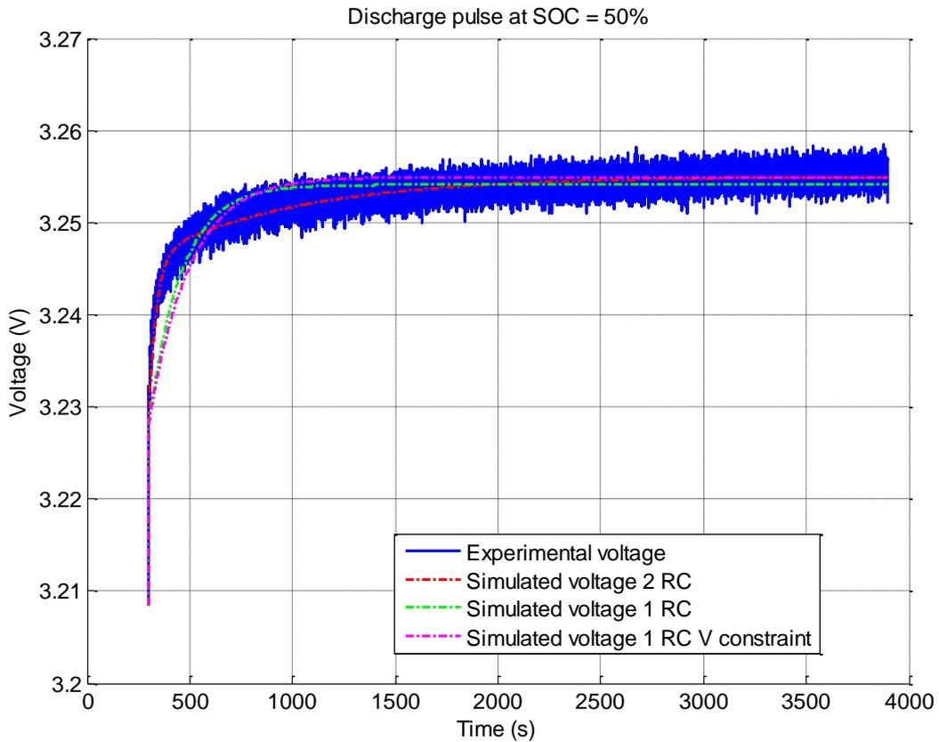
Figure 6. Voltage behaviour immediately after the end of a discharge process, while SOC=50%.
