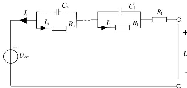
Figure 1. Generic structure of electric model of lithium cell (1<sup>st</sup> form).
