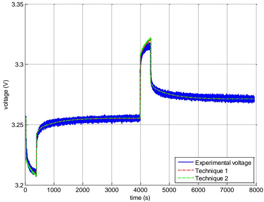
Figure 10. Comparison of voltage behaviour of models whose R-C parameters are evaluated with mean value charge/discharge (tech. 1) or global optimisation (tech. 2).
