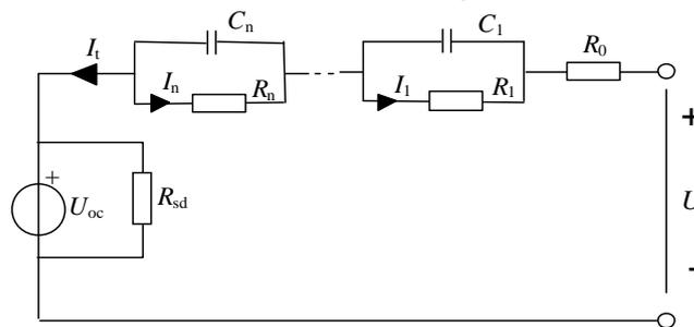
Figure 4. Model of Figure 1 with the addition of the self-discharge resistance  $R_{sd}$ .
