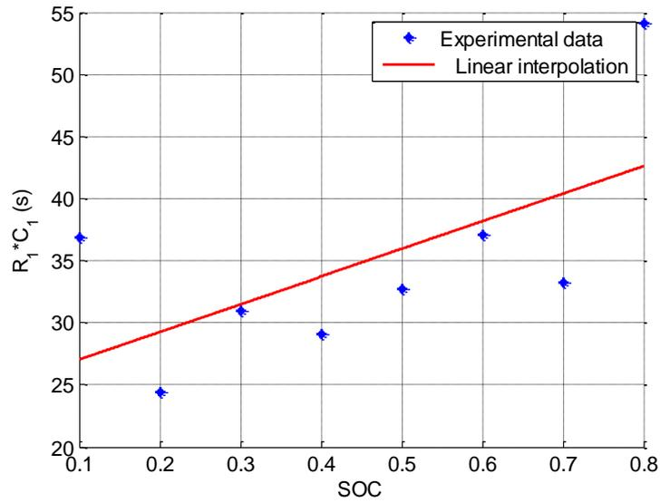
Figure 16. Experimental data on time constant  $R_1C_1$  and linear interpolation.
