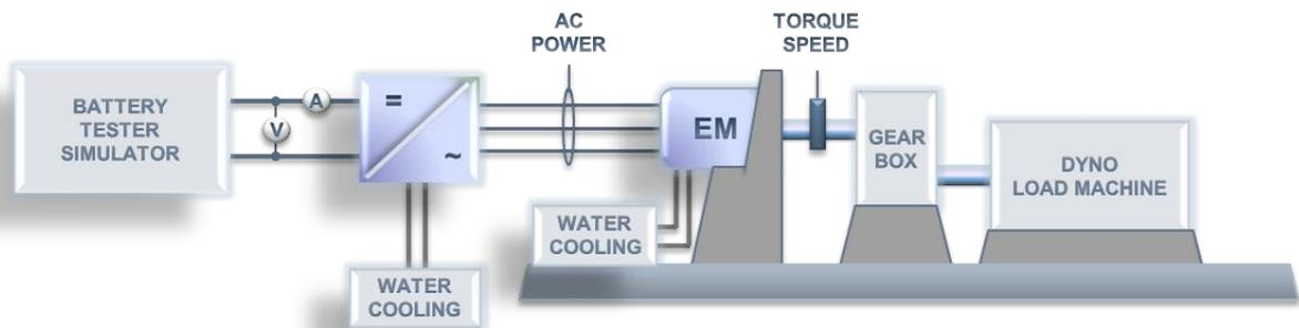
**Figure 4 Test setup of electric motor (EM) and its inverter (=/~)**
