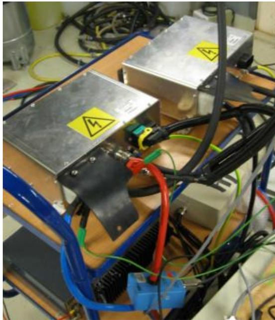
**Figure 2 DC/DC test setup**
