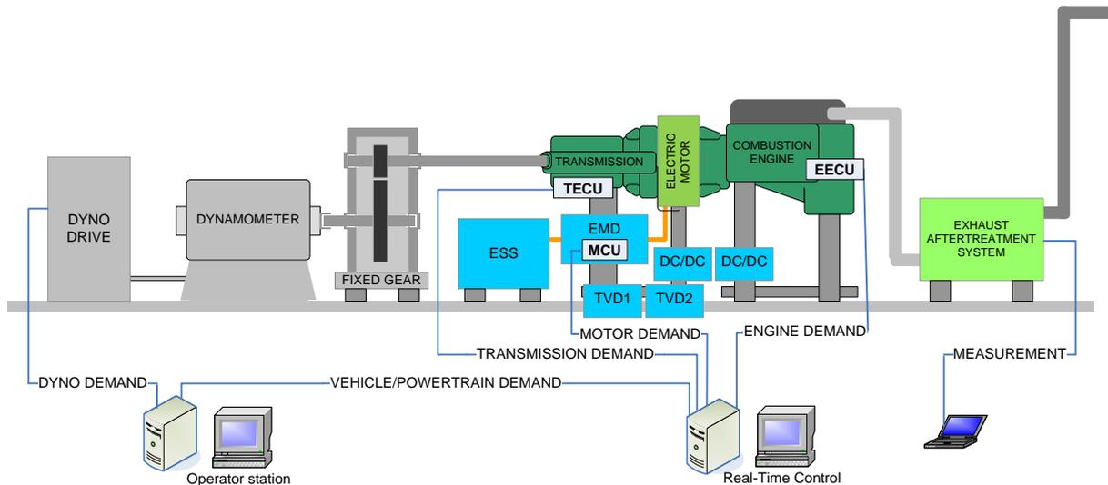
**Figure 6 Driveline rig test set up with combustion engine, transmission (gearbox), dynamometer and the hybrid components (ESS, electric motor, EMD).**
