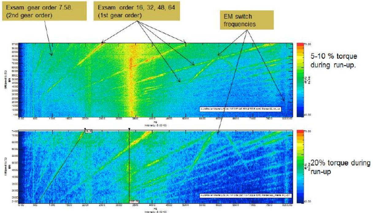
**Figure 9 Sound intensity spectra for two run-ups.**
