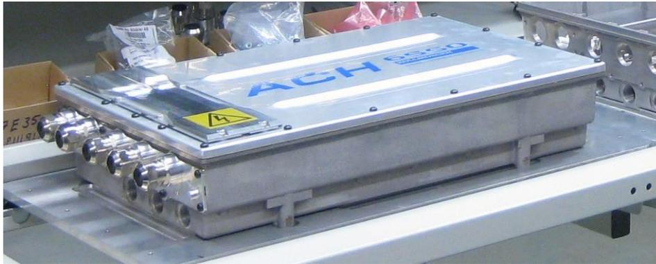
**Figure 5 Prototype inverter**
