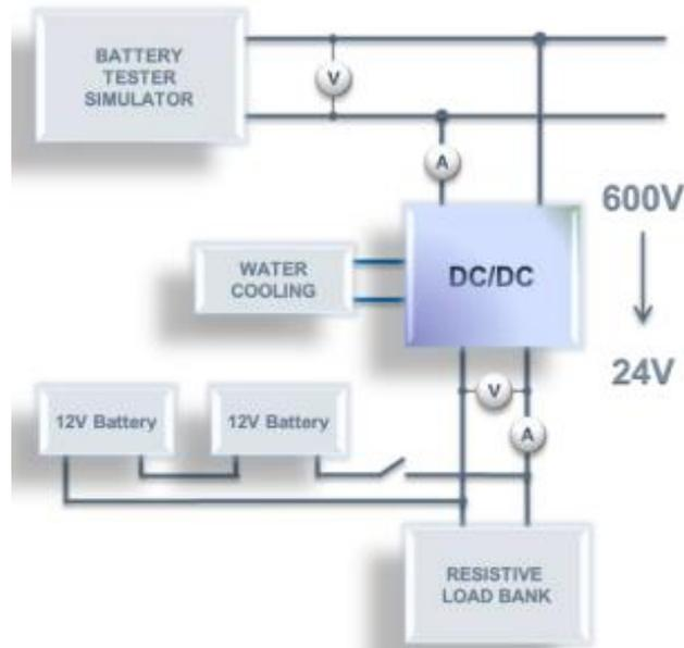
**Figure 3 DC/DC unit test setup**
