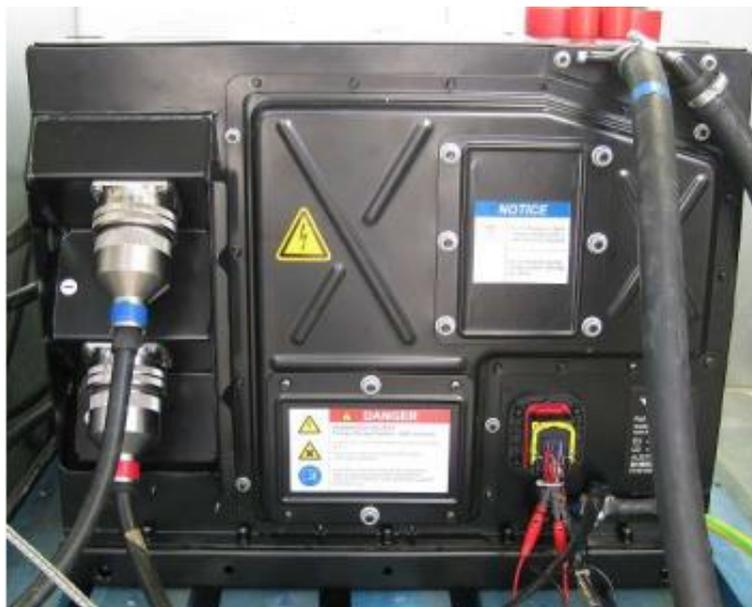
Figure 1 Energy storage system prototype for the HCV bus
