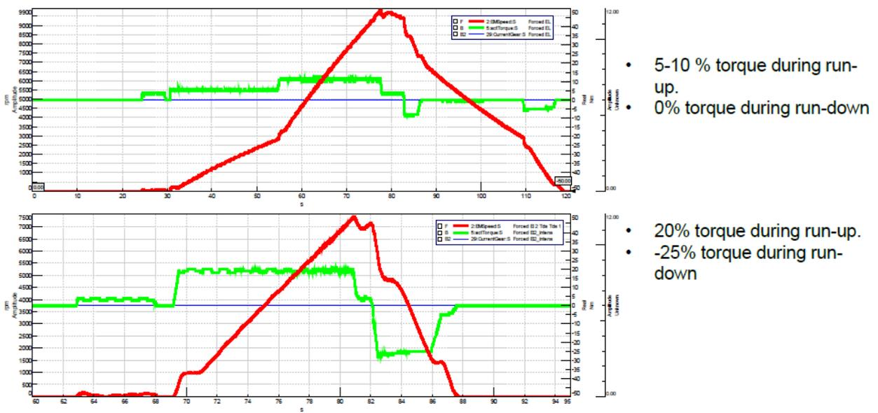
Figure 8 Two test cases for noise, showing speed, torque and gear.
