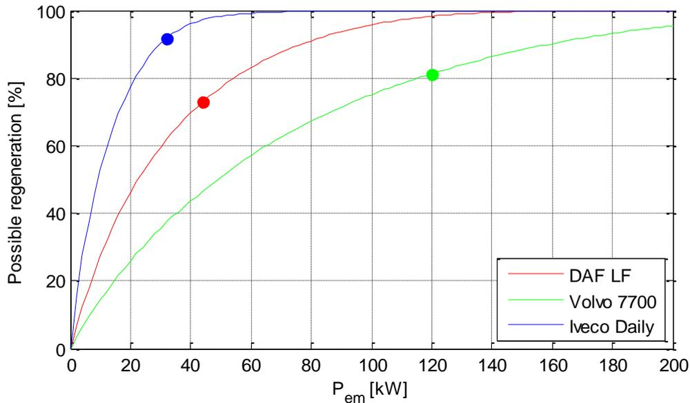
**Figure 11 Electric machine power rating versus energy recuperation capability**
