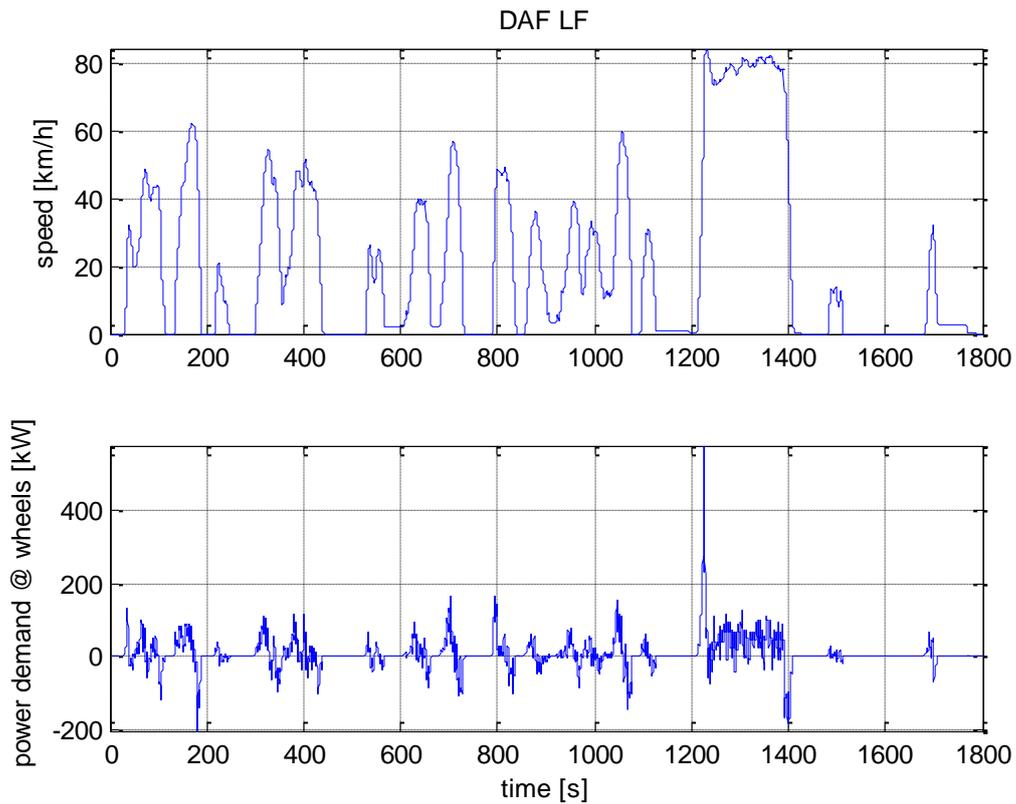
**Figure 5 DAF cycle and corresponding power demand at the wheels**
