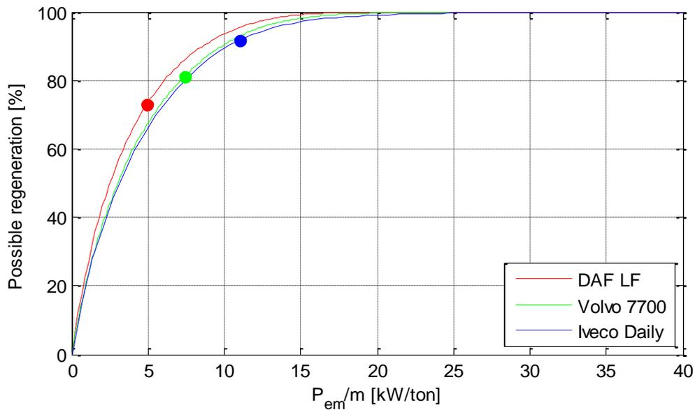
**Figure 12 Electric machine power rating normalized by vehicle mass versus energy recuperation capability**
