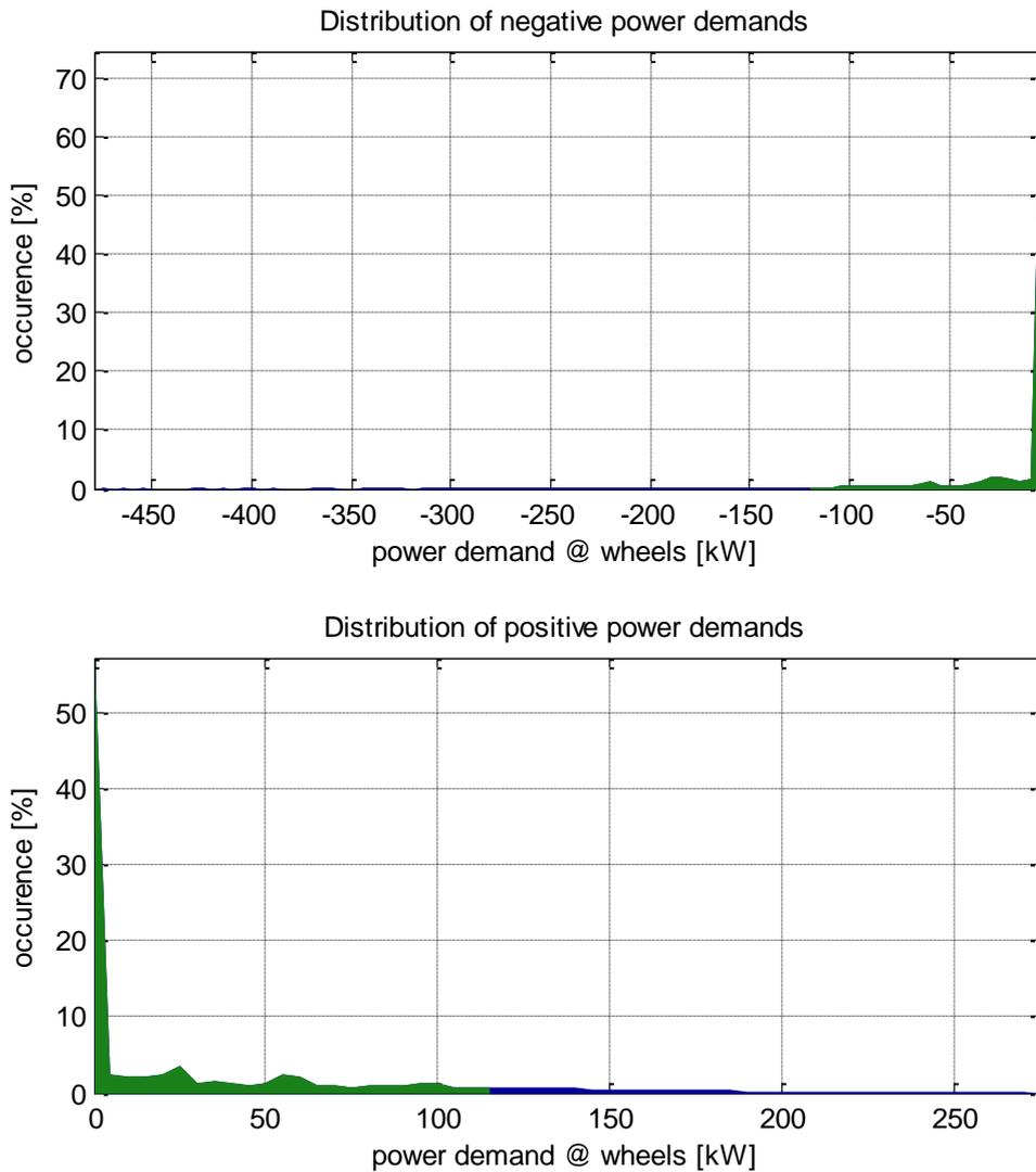
**Figure 8** Distribution of negative power demand at the wheels. The part indicated in green visualizes the capability of the electric machine in the Volvo 7700.
