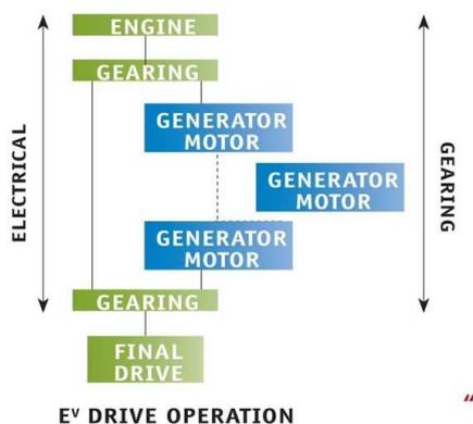
Figure 1: Series-parallel power split device of Allison, source <http://www.allisontransmission.com> 2010-04-21
