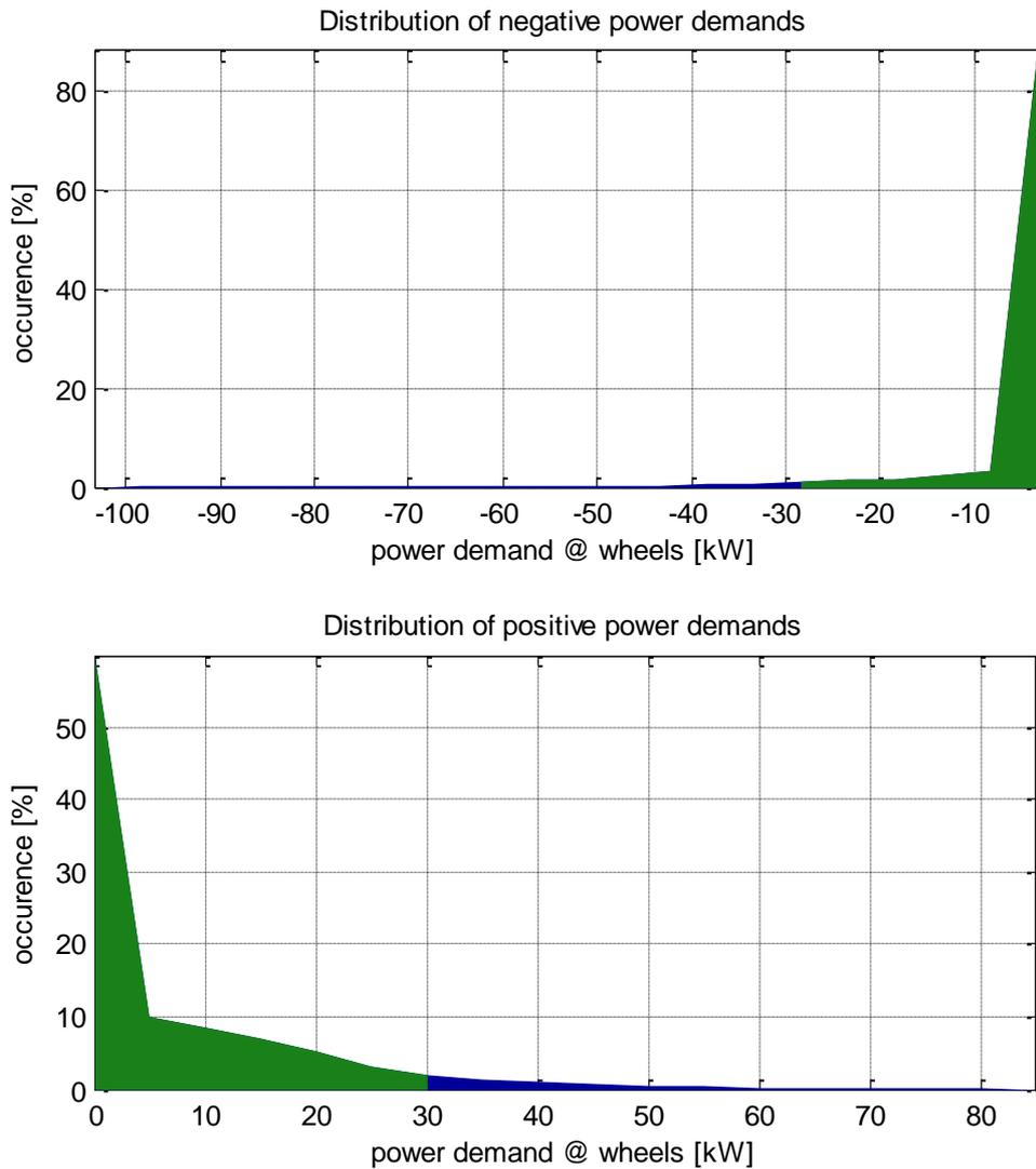
**Figure 10** Distribution of negative power demand at the wheels. The part indicated in green visualizes the capability of the electric machine in the Iveco Daily.
