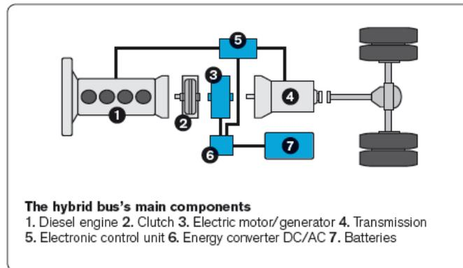
**Figure 2: Parallel hybrid power split of Volvo, source Factsheet Volvo 7700 hybrid EN.pdf 2010-04-21**
