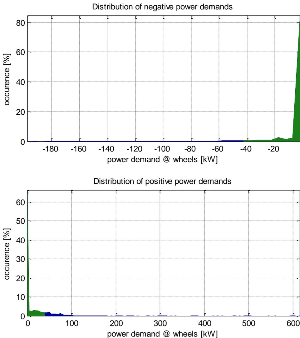
**Figure 6 Distribution of negative power demand at the wheels. The part indicated in green visualizes the capability of the electric machine in the DAF LF.**
