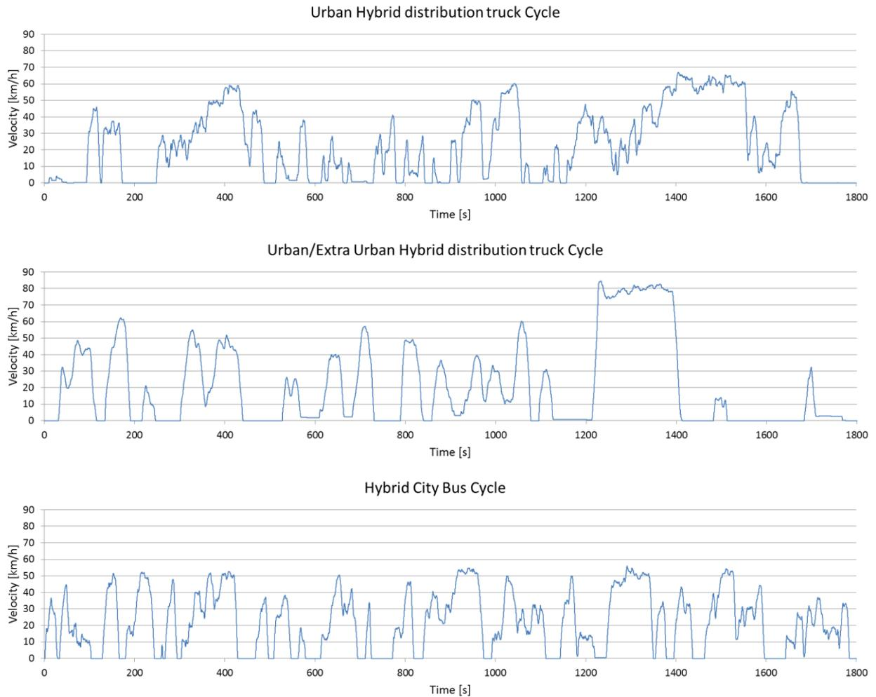
**Figure 3: Developed drive cycles by TNO in the HCV project**
