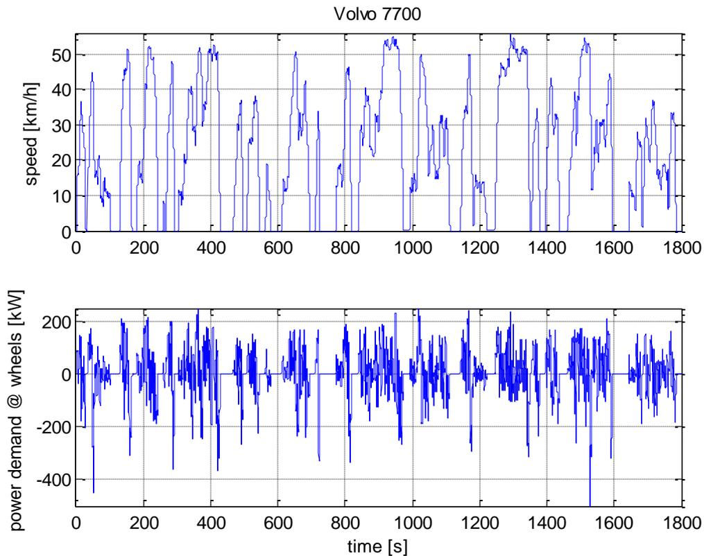
**Figure 7 Volvo cycle and corresponding power demand at the wheels**
