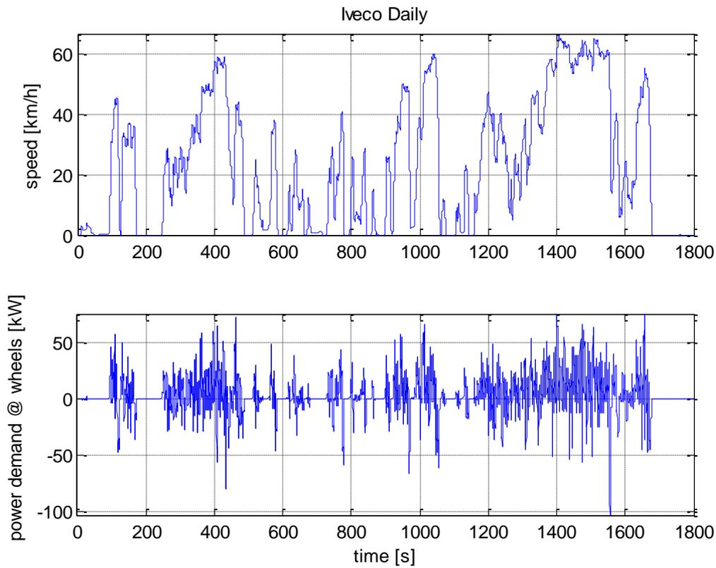
**Figure 9 Iveco cycle and corresponding power demand at the wheels**
