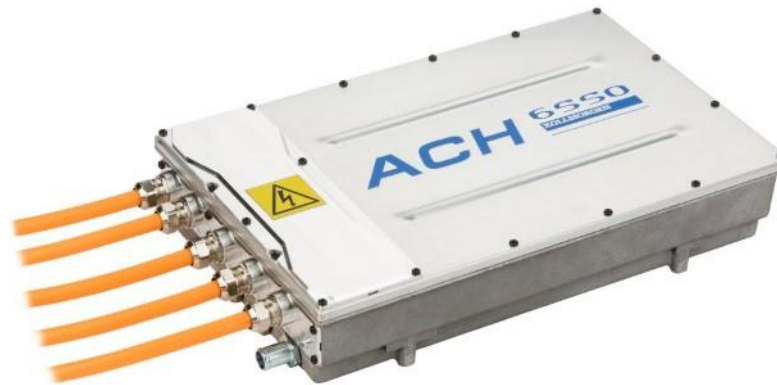
ACH 6550 Si, DC/AC converter, WEG cooled, 750 VDC, 550 ARMS peak
